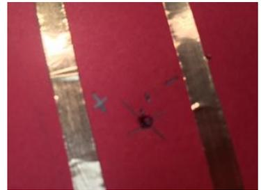
4. Cut two strips of copper tape, about the length of the parallel lines on your sketch. Peel and tape each strip to the lines on the paper.
